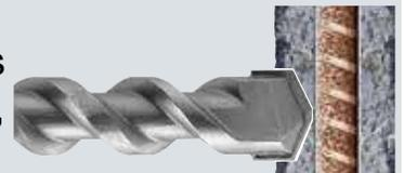
2. For drilling through rebar insert **RebarCutter™** into rotary hammer. Use rotary **hammer** mode. Apply firm pressure. When finished remove **RebarCutter™**.
